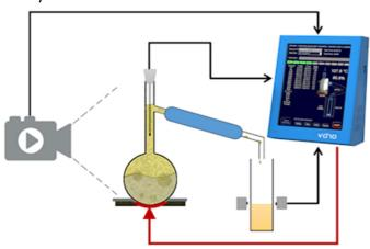
The entire test procedure is fully automated: position of the flask, temperature regulation of condenser and receiver, flask heating control, measuring vapor temperatures and volume, detecting IBP and FBP, rate control, barometric correction and recording all data. At test completion, the heater is automatically lowered and flask cooled down quickly. Results are displayed, saved, printed, sent to LIMS or USB.
